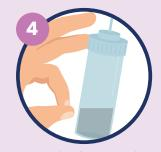
Close the vial with the provided cap and push firmly onto the vial.
